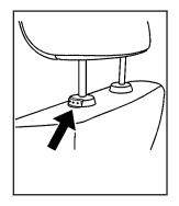
Pull up on the head restraint to raise it. To lower the head restraint, press the button located on top of the seatback and push down on the head restraint.
